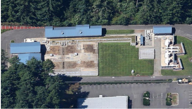
LACEY WA - LOTT Satellite Martin Way RRP, ADWF Capacity 7.6 MLD existing, 18.9 MLD ultimate design
