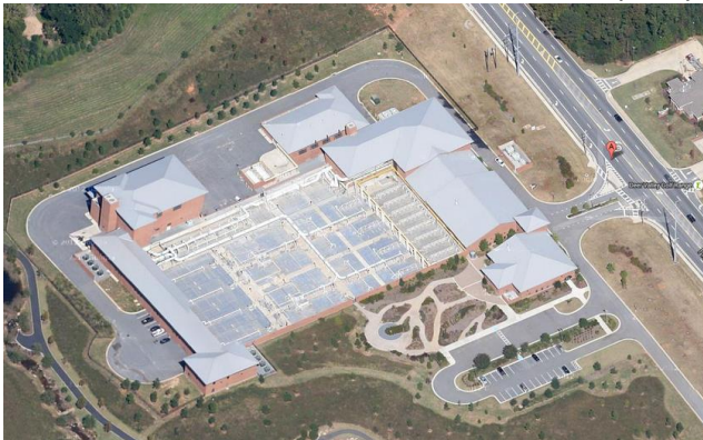
FULTON COUNTY GA – Johns Creek EC, AAF Capacity 45 MLD existing, 61 MLD future
