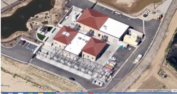
SANTA PAULA CA – WRF, ADWF Capacity 13 MLD existing, 16 MLD design
