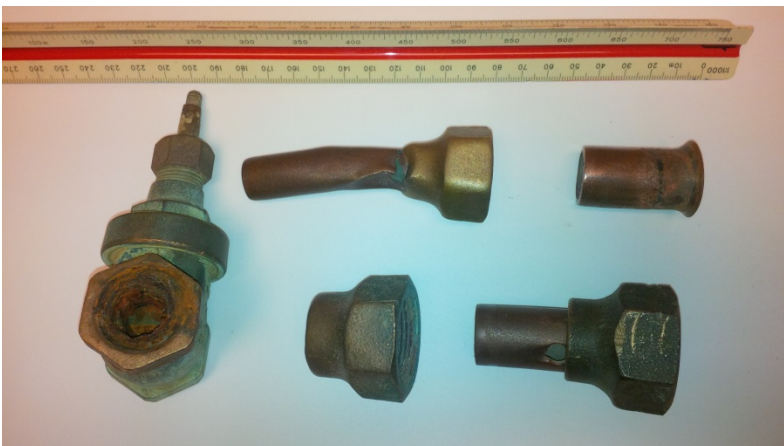
Photo 2 – variety of damaged fittings
