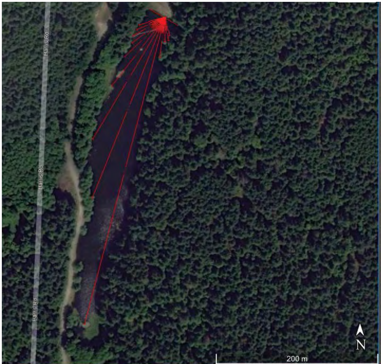
Figure 3: Radials used to calculate the effective fetch length
