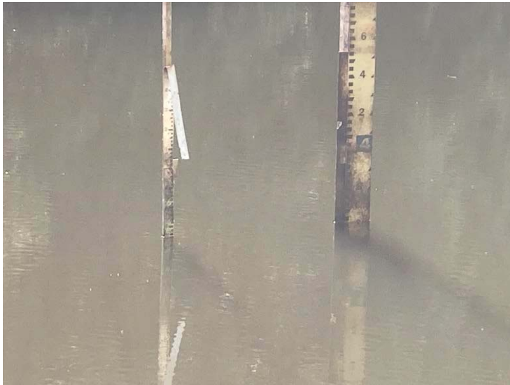
Photo 3: Staff gauges – difficult to read. (2022-08-31, JDM)
