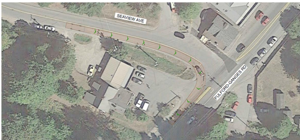
Analysis of 40-foot tour bus turning movements if turning left onto Fulford-Ganges Road from Seaview Avenue (which continues on from Jackson Avenue and the proposed tour bus parking option located there).
