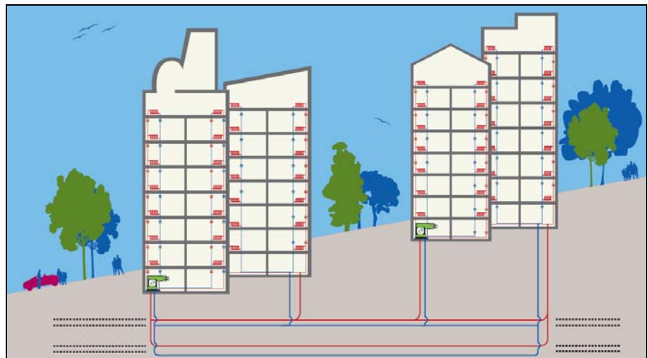
Figure 11: Lonsdale Energy Corp. District Loop Illustration
