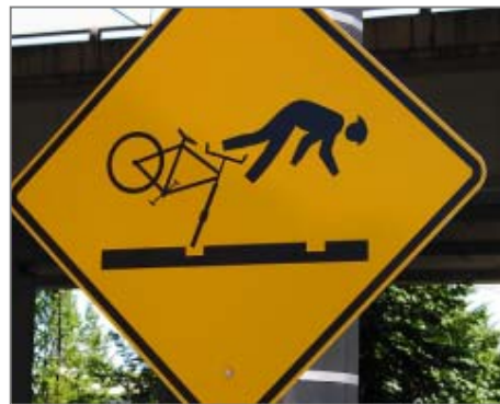
Figure 6. Signs alert cyclists that they are approaching tracks and direct them to approach the tracks at a near 90° angle.
